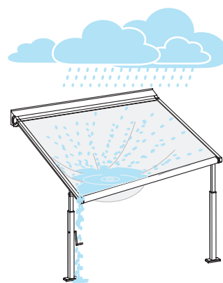
When exceeding rain class 2 (56 l/h/m 2 ), the Plaza Viva must be retracted. Risk of damage!
